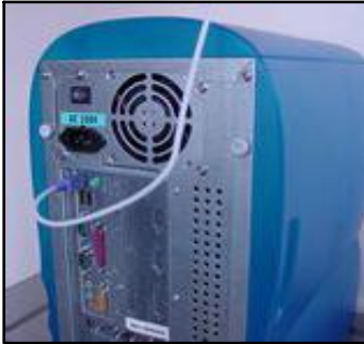
(U//FOUO) Pre-installation: standard cable connects the keyboard to the PS/2 processor port.
