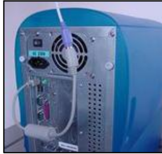
(U//FOUO) Post-installation: hardware keystroke logger inserted between keyboard and PS/2 processor port.
